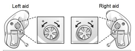
With the hearing aids in the ears, locate the volume wheel with the tip of a finger. For both right and left hearing aids:
